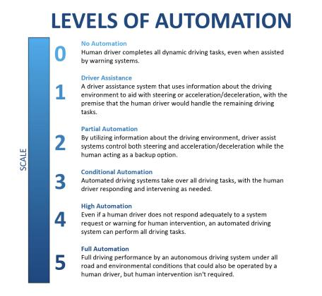
FIGURE 5 - THE SIX LEVELS OF DRIVING AUTOMATION ("A BRIEF HISTORY OF AUTONOMOUS VEHICLE TECHNOLOGY," 2016)
