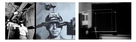
FIGURE 3: SPROUL'S HEAD-MOUNTED DISPLAY TO PROJECT VIRTUAL IMAGES (BASU, 2019)
