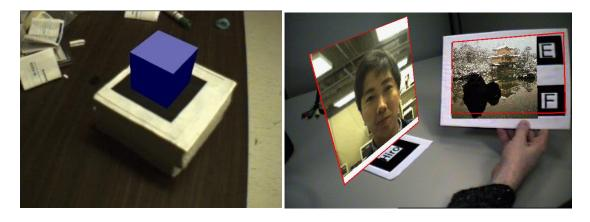
FIGURE 8: AR TOOLKIT TO CREATE: LEFT – SIMPLE VIRTUAL BLOCK ALIGNED WITH A PHYSICAL OBJECT; RIGHT – REMOTE CONFERENCING OPTION (KATO, BILLINGHURST, BLANDING, & MAY, 1999)
