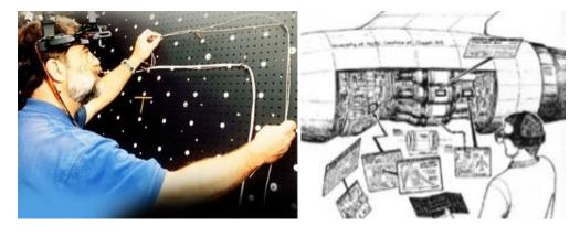
FIGURE 5: HEADSET FOR BOEING CO. TO VIRTUALLY DISPLAY FIXTURES OF AN AIRPLANE (RIVES, 2018)
