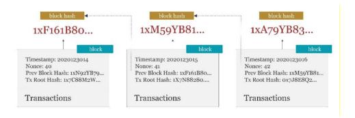
FIGURE 1. BLOCKCHAIN STRUCTURE (KHATIB ET AL., 2021).
